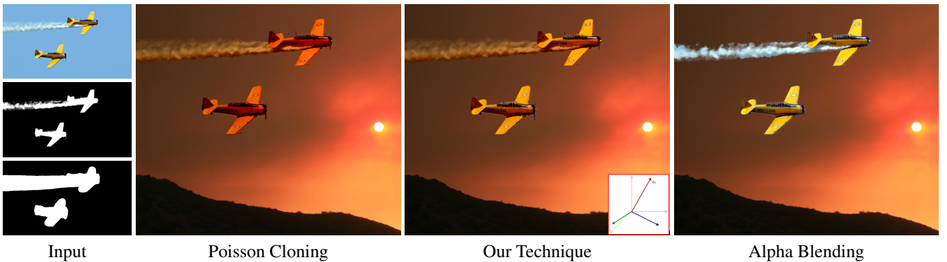
Figure 9: Image composition of two planes into a sunset background. (first column) Input: source image, alpha mask, and pasting mask, respectively. The remaining columns show compositing results obtained using Poisson cloning, our method ( w = (0.55, 0.63, 0.64) ), and alpha blending. Our method diffuses the background color over the inserted patches, simulating the effect of ambient illumination. Note the colors of the planes and of the steam. The inset shows the new basis \mathbf{B} .
